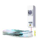
Checking the amount of linearity & deflection of optical disk or spindle motor. By using a featured HIP-1000's "Orbital measurement" function, the central point of rotation deflection can be observed with real time measuring of orbital tracking.
