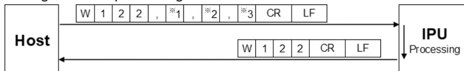
\*1: Data output mode  ("0"=Stream, "1"=I/O input, "2"=OFF)
