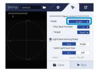
4 Set the number of measurement spots with [Max Spot Number], and set the judgment target spot with [Target].
