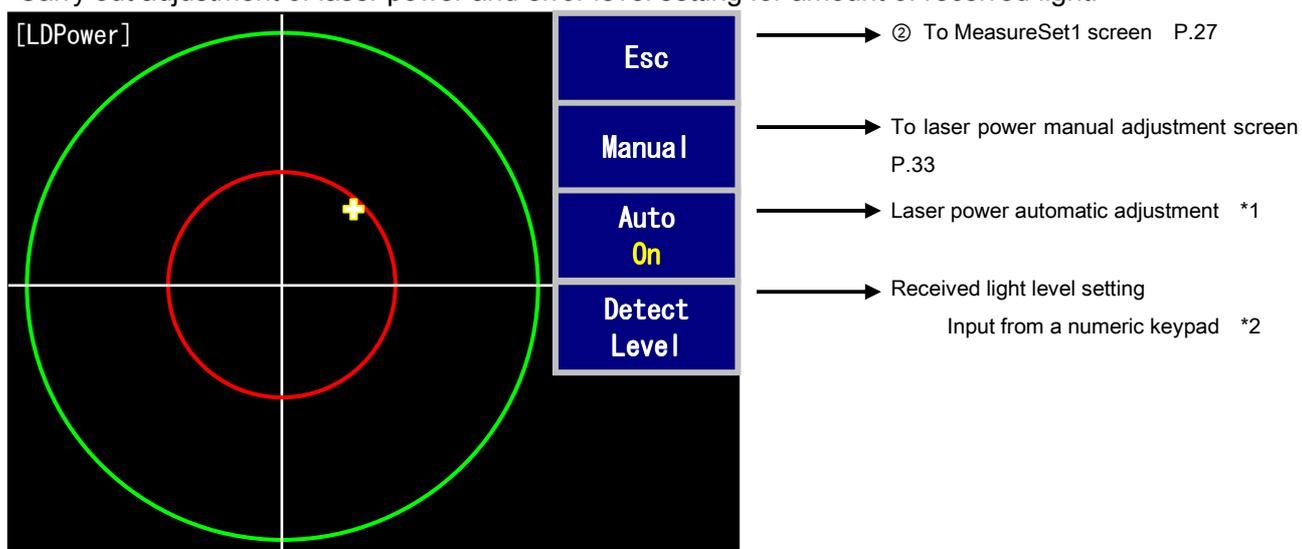
\*1 If the laser power automatic adjustment is set to ON, the adjustment is carried out automatically when the measurement is started.
