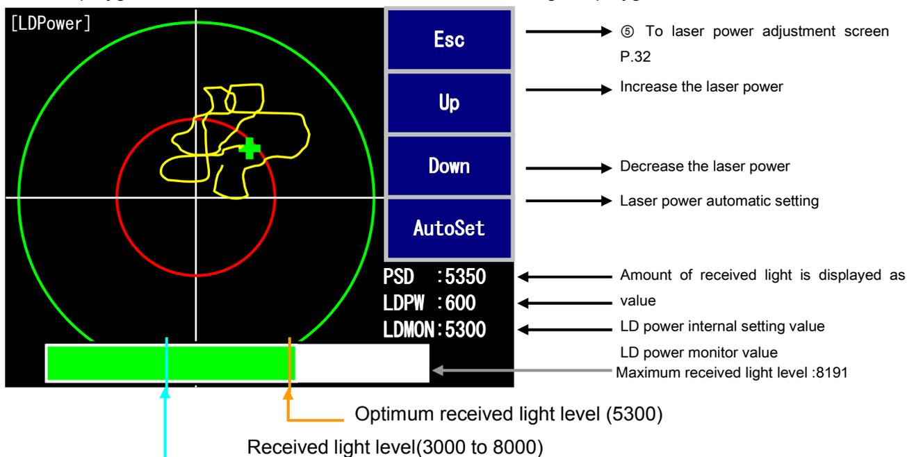
\* The amount of received light can be measured if the level bar is green, however, set it to approximately 5300 as an optimum value (refer to the figure above).
