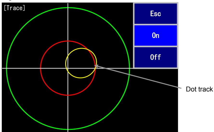
\* If the standard measurement is changed to the motor measurement, the trace function is automatically set to On.
