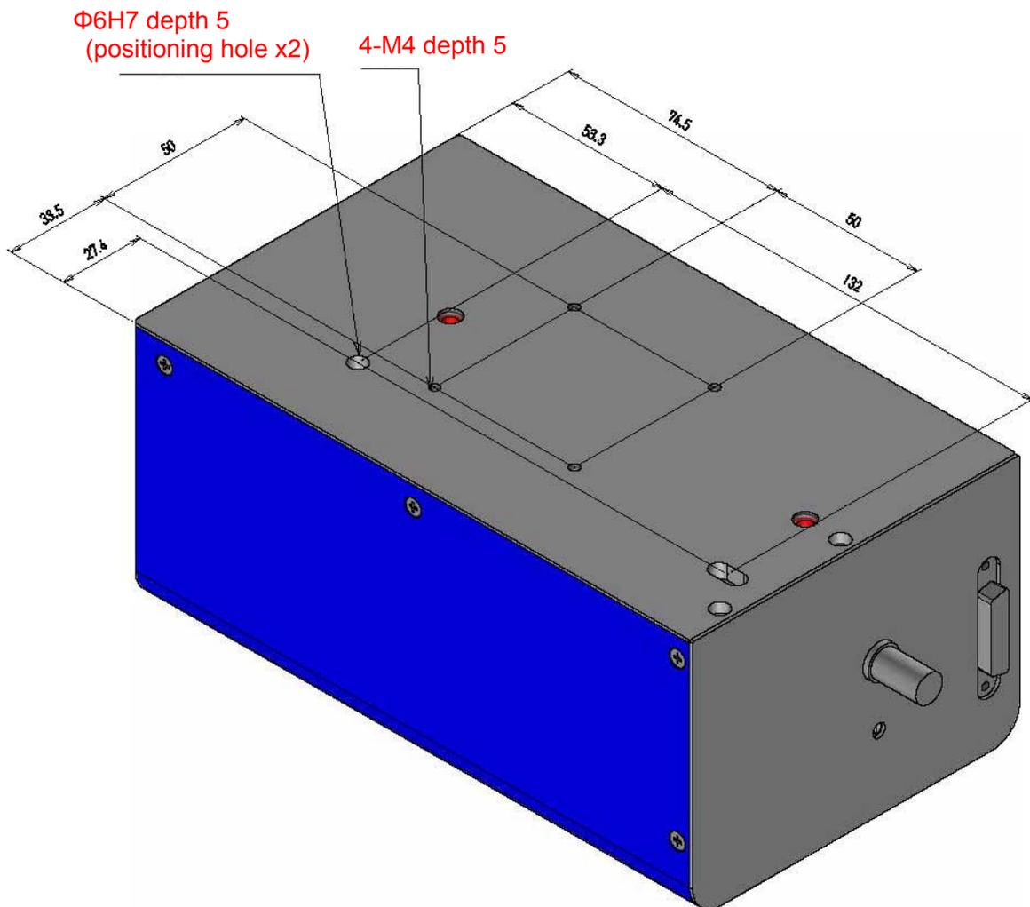
**Figure 8. Attachment dimension diagram**
